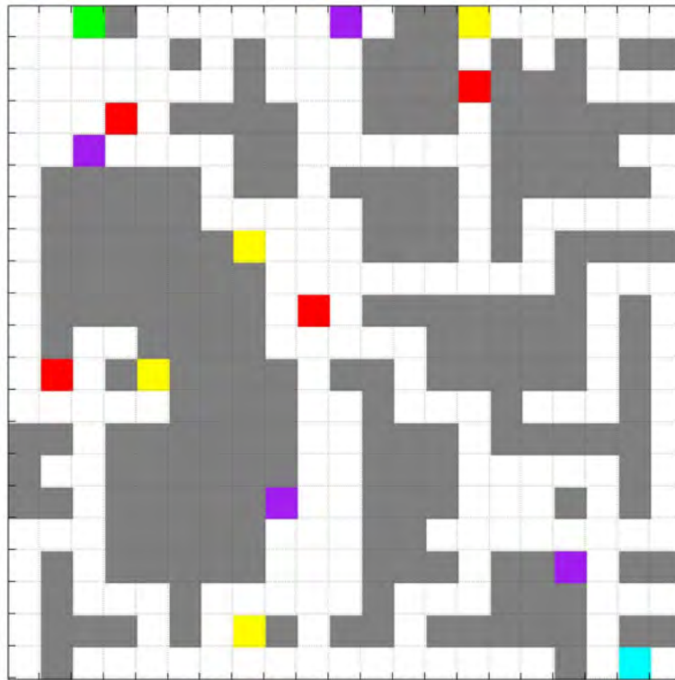
Figure 1: Example of the Arena. Walls are marked with grey squares. Yellow squares mark the drop-off points, purple squares mark the pick-up points, red squares mark the hazard points, green and cyan squares mark the entrance and exit, respectively.
